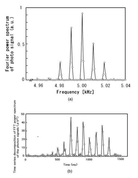
FIG. 4. A. FFT spectrum of the whole photo signal shown in Fig. 3(B). (data length: 1second) B. Time series decomposition of the FFT power spectrum of the photon signals. The intervals of the plots are 10ms. Each plot is the peak value of the FFT power spectrum at 5kH for the data length of 10ms.
