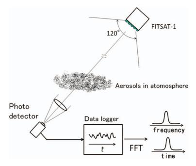
FIG. 2. Configuration for detection and identification system of the LED light signal using Fourier analysis.
