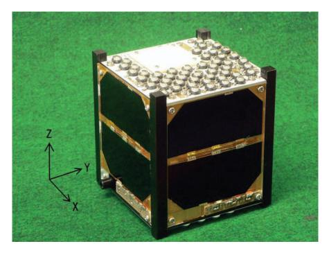
FIG. 1. A small cube satellite (code name: FITSAT-1, nickname: "NIWAKA"). 50 high brightness LEDs are installed on the top surface (z surface).
