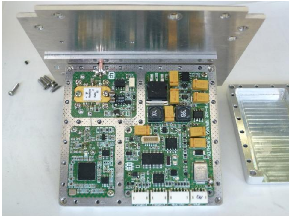
Inside view of 5.8GHz TX
