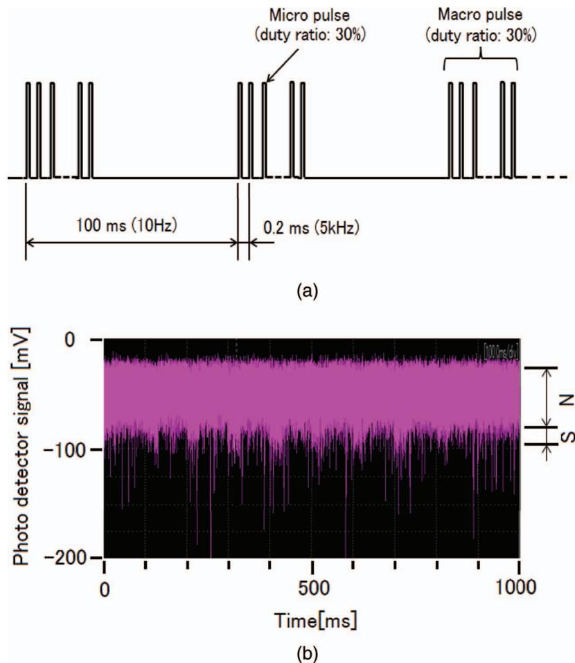
FIG. 3. A. Temporal configuration of the LED emission signal. The signal consists of the continuing macro pulse train of 10 Hz (duty ratio: 30%), and each macro pulse is modulated at 5 kHz and consists of 150 micro pulses. Whole length of the pulse train is 120 second. B. Output signal of the photo detector recorded by the data logger. (S: signal, N: noise) The data were taken at 1:10 on Dec. 14th (Japan standard time) in Yufu city, Fukuoka prefecture, Japan.
