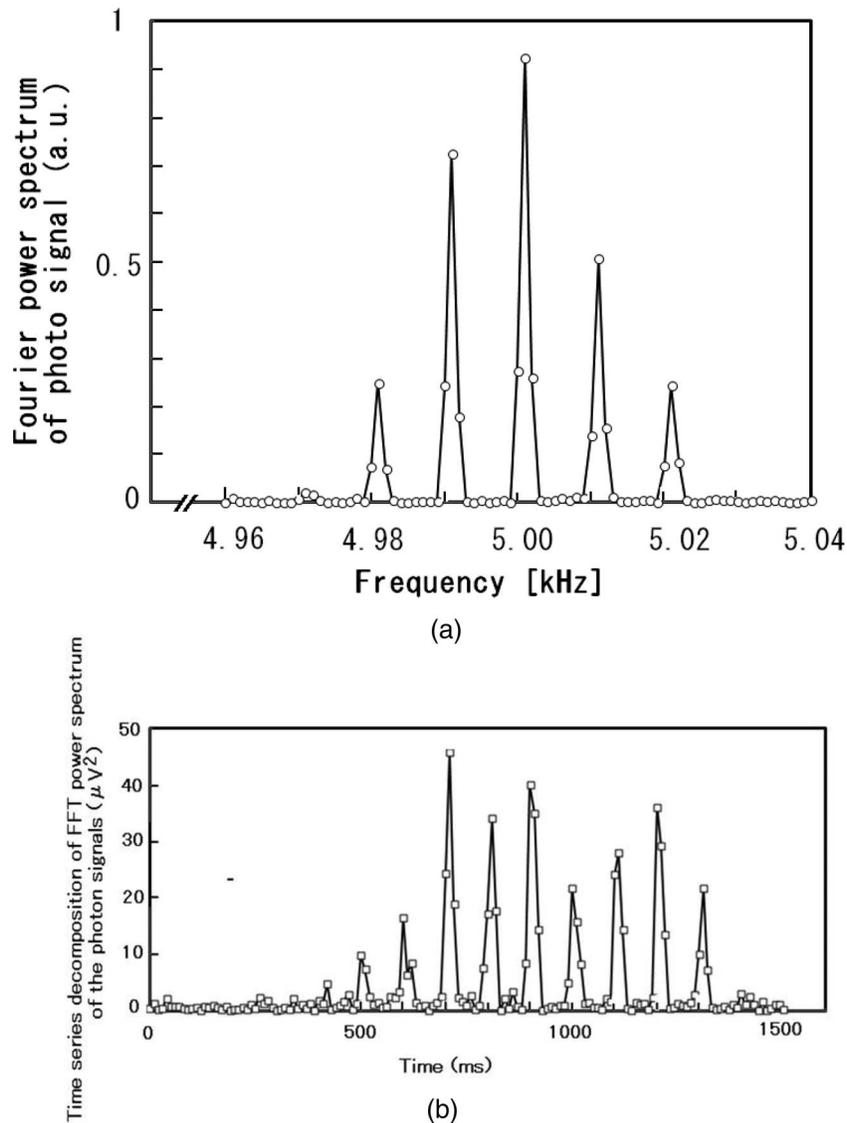
FIG. 4. A. FFT spectrum of the whole photo signal shown in Fig. 3(B). (data length: 1second) B. Time series decomposition of the FFT power spectrum of the photon signals. The intervals of the plots are 10ms. Each plot is the peak value of the FFT power spectrum at 5kHz for the data length of 10ms.
