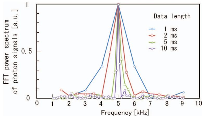
FIG. 5. FFT spectrum of signal of the photo detector. Even for the data length of 1ms, the spectrum peak at 5kHz can be clearly seen.
