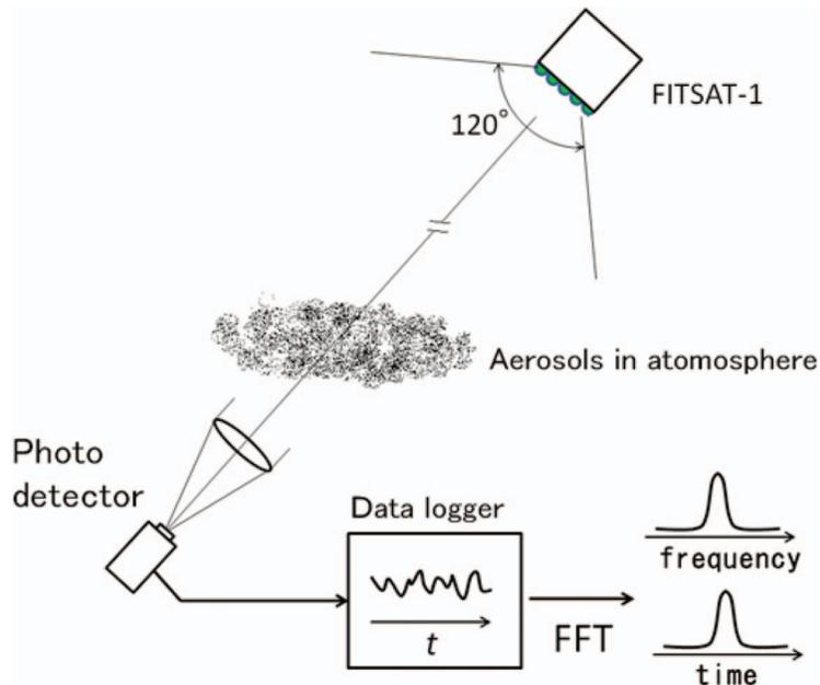
FIG. 2. Configuration for detection and identification system of the LED light signal using Fourier analysis.
