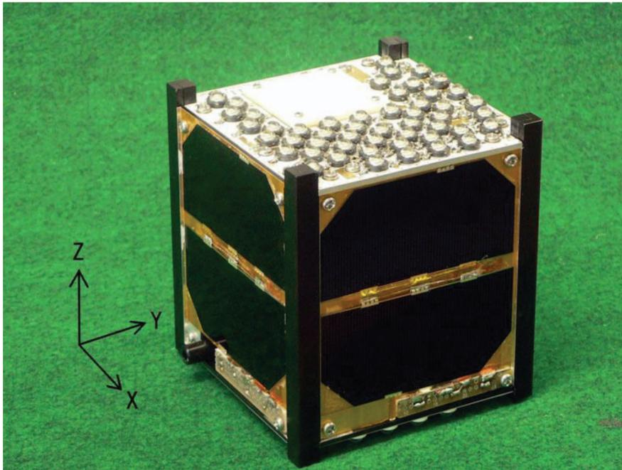
FIG. 1. A small cube satellite (code name: FITSAT-1, nickname: "NIWAKA"). 50 high brightness LEDs are installed on the top surface ( $z$  surface).
