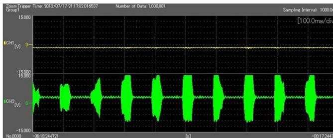
Fig. 10. Comparison of LED signals without (upper signal) and with (lower signal) the band path amplification. Horizontal full scale is 1 [s] and both vertical full scales are 30 [V].
