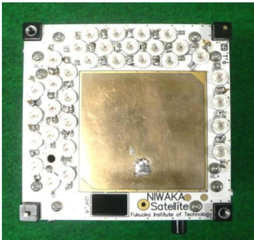
Fig. 3. Front panel of FITSAT-1 equipped with LEDs.
