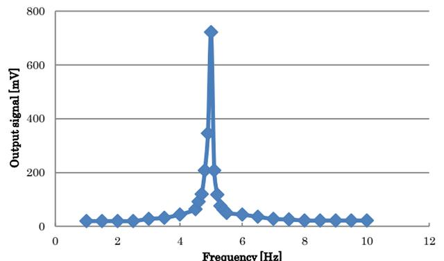
Fig. 9. Amplification characteristic of the sinusoidal wave of 2 [mV].
