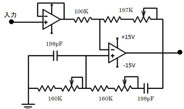
Fig. 8. Electronic circuit of the active band-path filter.
