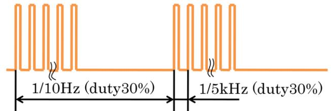
Fig. 4. Temporal construction of the LED signal.
