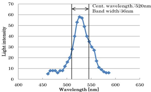
Fig. 7. Wavelength spectrum of the green LED with the band width of the optical band path filter.
