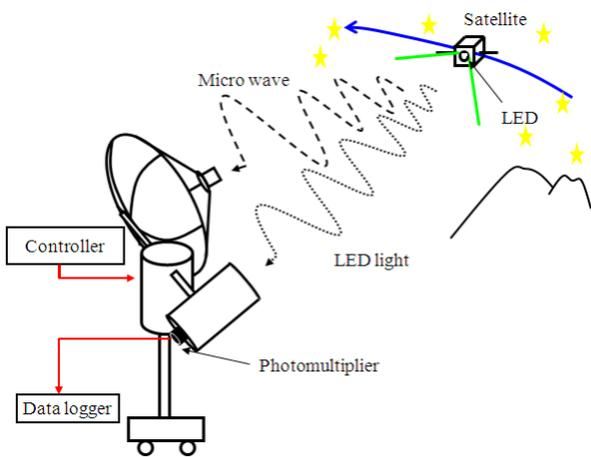
Fig. 2. Overview of the experimental system.
