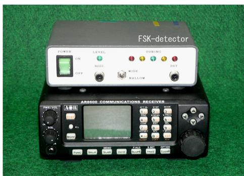
Fig. 25. AR8600 receiver and FSK detector.
