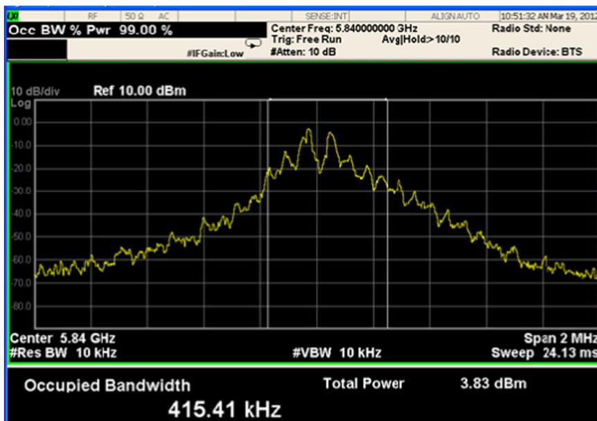
Fig. 19. Spectrum of 5.84 GHz signal.
