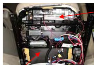
bearing plate linear actuator Seat yaw DOF added to car seat to provide spine rotation
