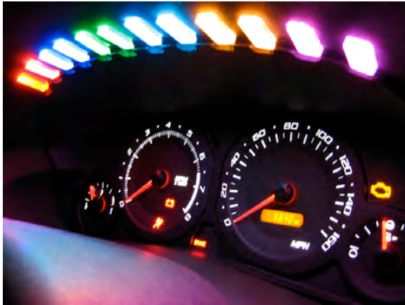
Main navigational array of Stanford lighting system that communicates turn direction and distance to turn through dynamic effects
