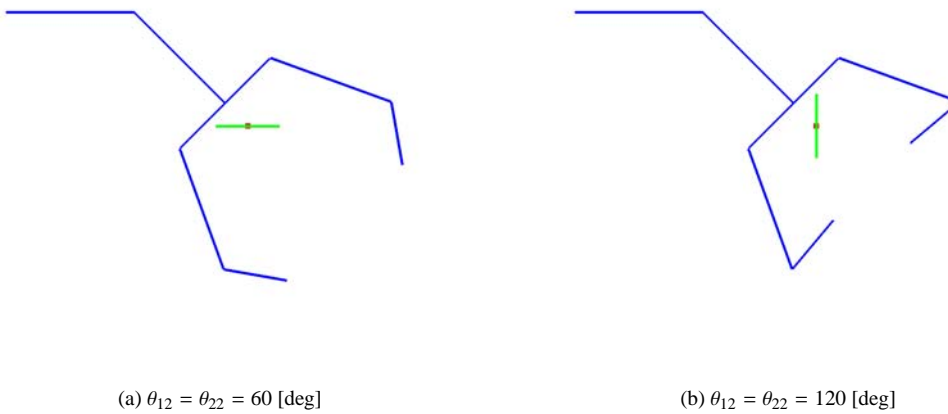
Figure 16. Illustration of partial caging for a stick-shaped object.
