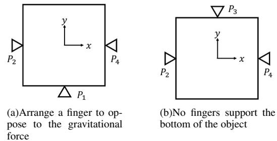
Fig. 1 Grasping by three-fingered hand in two-dimensional space. Gravitational force is applied toward  $-y$  direction.
