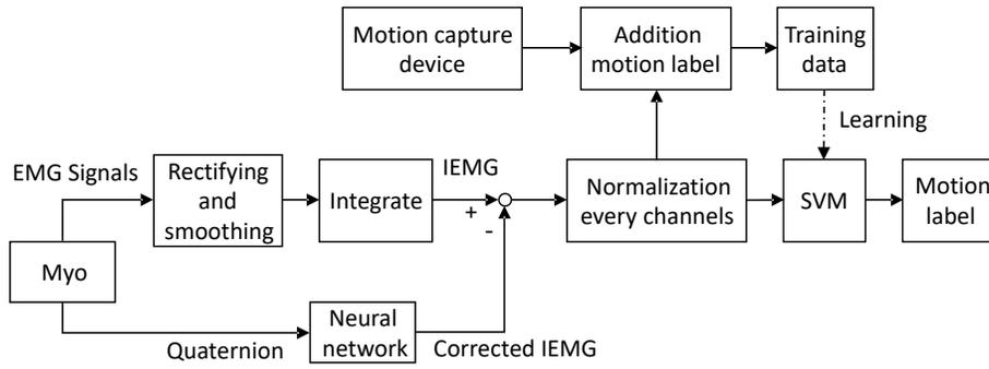
Fig. 9. A correction diagram for upper limb posture
