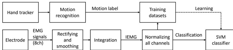
Fig. 3. A classification diagram for the six hand states
