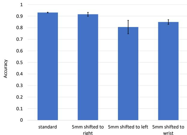
Fig. 5. Location changing interfere with classification accuracy
