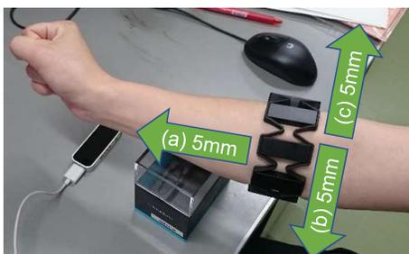
Fig. 4. Offset of sensors alignment
