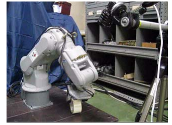
Fig. 12. Caging the cylinder by the arm/hand system
