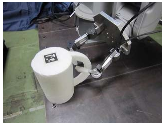
Fig. 14. Experiment: Caging the mug-like object
