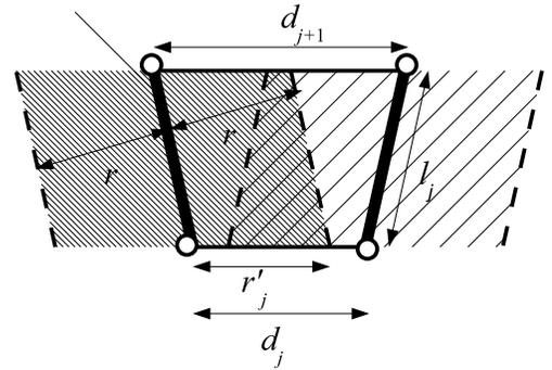
Fig. 5. C-obstacles cover completely the face formed between both finger bodies
