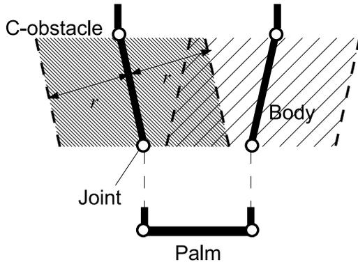
Fig. 4. C-obstacles of finger bodies in the case of caging a sphere
