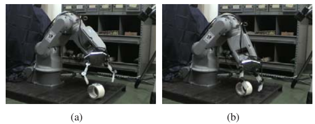
Figure 22 A failure case of planned caging motion caused by any collisions (the object moved)
