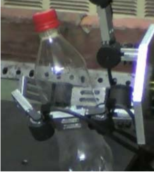
Figure 3 Caging a bottle (Waist-type caging)
